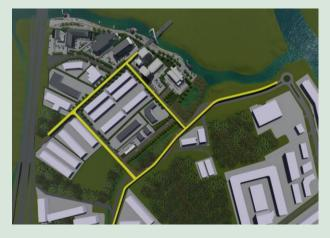
The construction of Loop Road Phase 4, designed with a width of 40 meters, will connect the existing developments in Kiulap Phases 1, 2, and 3. This project is expected to enhance traffic flow and alleviate congestion in the area. Additionally, internal roads with widths of 15 meters and 20 meters will be constructed to facilitate connectivity between future developments within this planning scheme.
